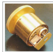
Figure 6 — Photo of a 50 W HF Element lower level showing a similar Bruene pickup.
